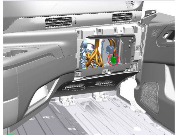
The location of the upfit connector located in the fusebox room
